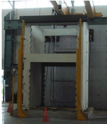
Figure 1.1. Full scale HCPS model for lateral cyclic loading test (Tiong et al , 2013)
