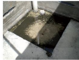
Fig. 5: Waterproofing test. Top floor with water (left). Bottom floor without leakage (right)
